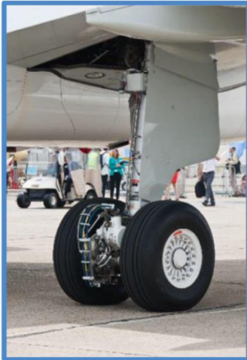
Figure 8: An onboard technology taxi system (electric green taxi system - EGTS) as presented during Paris Air Show 2013
