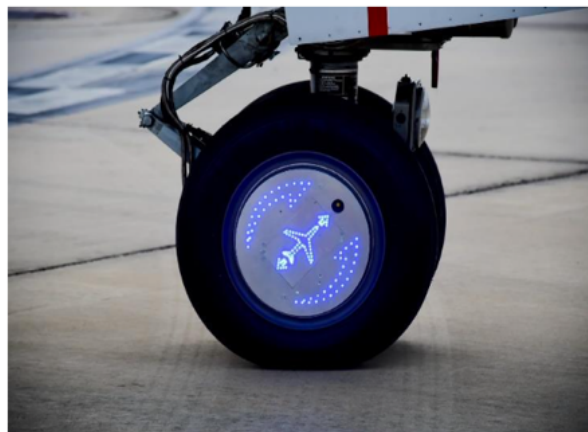
Figure 9: An onboard technology taxi system (Wheel Tug)
