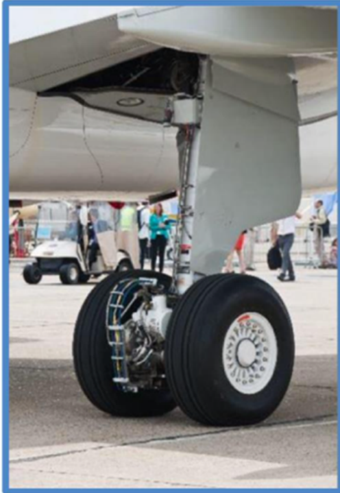
Figure 8: An onboard technology taxi system (electric green taxi system - EGTS) as presented during Paris Air Show 2013
