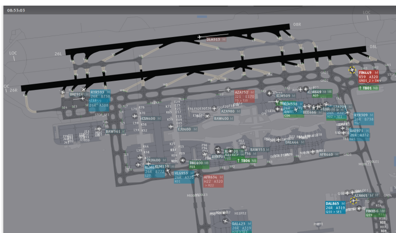
Figure 17: A-SMGCS used in conjunction with our interfaces.
