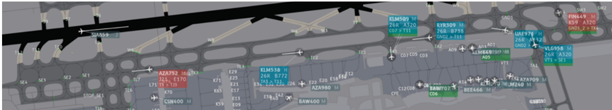
Figure 3: Main radar image for supervising moving aircrafts on the airport (Paris-Charles de Gaulle here). Blue labels correspond to departing aircrafts and red label to arriving aircrafts. Green labels represent towing vehicles.
