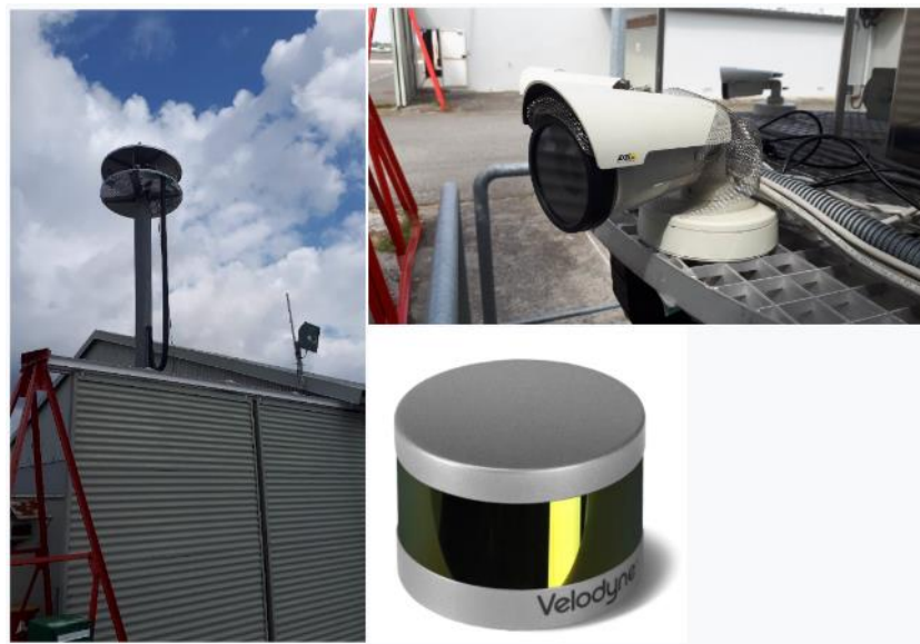
Figure 12 Cameras and LIDAR from the Muret airfield
